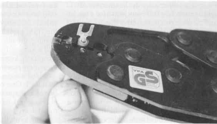
Figure 3-45. A ratcheting-type crimper that does a perfect job every time. This one makes a double crimp (see Figure 3-46).
