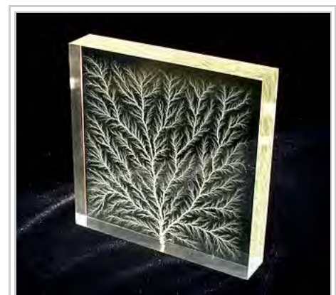
Dielectric breakdown within a solid insulator can permanently change its appearance and properties.
