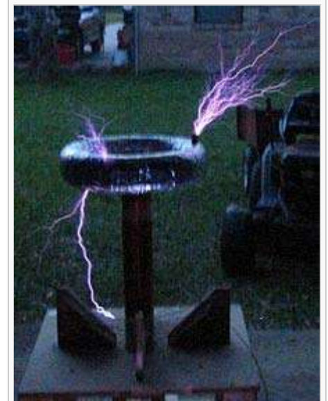
A small, later-type " Tesla coil " in operation. The output is giving 17-inch sparks. The diameter of the secondary is three inches. The power source is a 10000 V, 60 Hz current limited supply.
