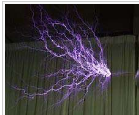
Electric discharge showing the lightning-like plasma filaments from a Tesla coil.
