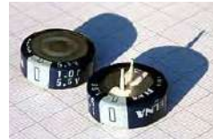
Typical button style supercapacitor for PCB mounting used for memory backup
