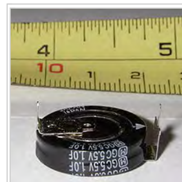
A 5.5 volt supercapacitor is constructed out of two single cells, each rated to at least 2.75 volts, in series connection
