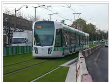
Supercapacitors are used to power the Paris T3 tram line on sections without catenary overhead wires and to recover energy during braking.
