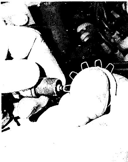
A spark plug's gap is correct if there is a slight drag on the proper size wire of the gauge.
