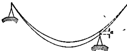
FIG. 48.—Error introduced by assuming constant equivalent span.
