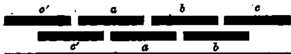
FIG. 79.—Sectional diagrammatic development of the phase belts of the winding of Fig. 78.
