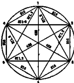
FIG. 20.—Diagram of converter voltages between collector-rings.
