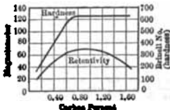
FIG. 31.—Hardness and retentivity of carbon-steel.
