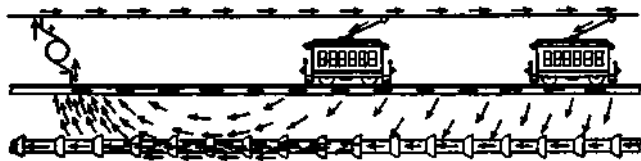
FIG. 131.—Conditions contributing to electrolysis.
