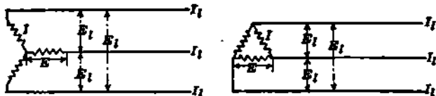
FIGS. 8 AND 9.—Internal and external e.m.f.s. and currents in three-phase alternators with Y and \Delta connections.
