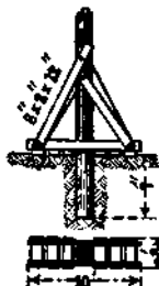
FIG. 47.—Methods of setting self-sustained poles.
