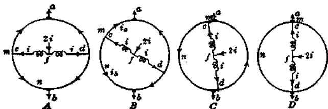
FIG. 24.—Relation between current and position of armature.
