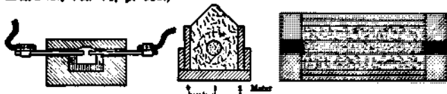
FIG. 1.—Moissan Arc Furnace. FIG. 2.—Acheson Carborundum Furnace.
