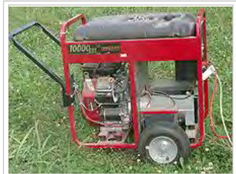
Electrical generator, with Generac Vanguard (Now Briggs Vanguard) engine and electric start
