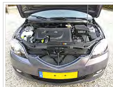
A Mazda3 with a modern common rail 1.6 liter turbodiesel engine (PSA) with variable geometry turbocharger, intercooler, 16 valves, double overhead camshafts and piezo controlled 7-stage direct injection.
