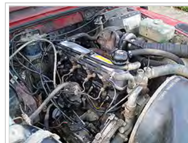
A Land Rover 2.5-litre 4-cylinder turbodiesel engine is typical of 'first generation' automotive turbodiesels, with mechanical indirect injection, 8 pushrod operated valves and no intercooler. The turbocharger itself is visible in the upper centre of this picture.
