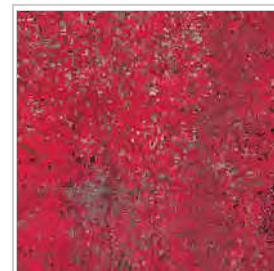
Infrared image of the above farms. Various colors indicate healthy crops (red), flooding (black) and unwanted pesticides (brown).
