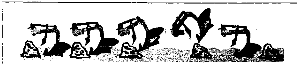
Fig. 26. Safety devices (protection against rocks and stumps) on a mouldboard plough.
