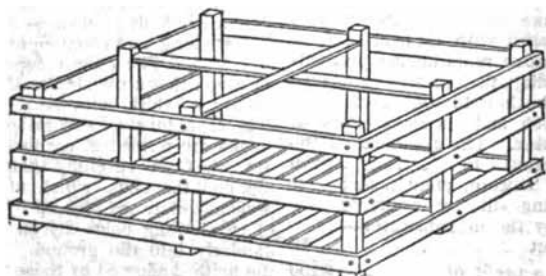
Frame in which the flax is packed to be steeped in the River Eys in Flanders.
