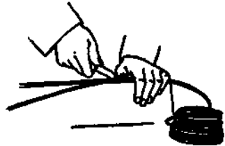
1. Cut off a sufficient length of fuse.
