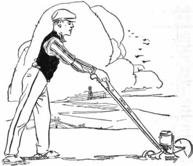
FIG. 114.—The wrong way to push a seeder or hand-cultivator. It is almost impossible to control the direction of the machine and the operator tires quickly.
