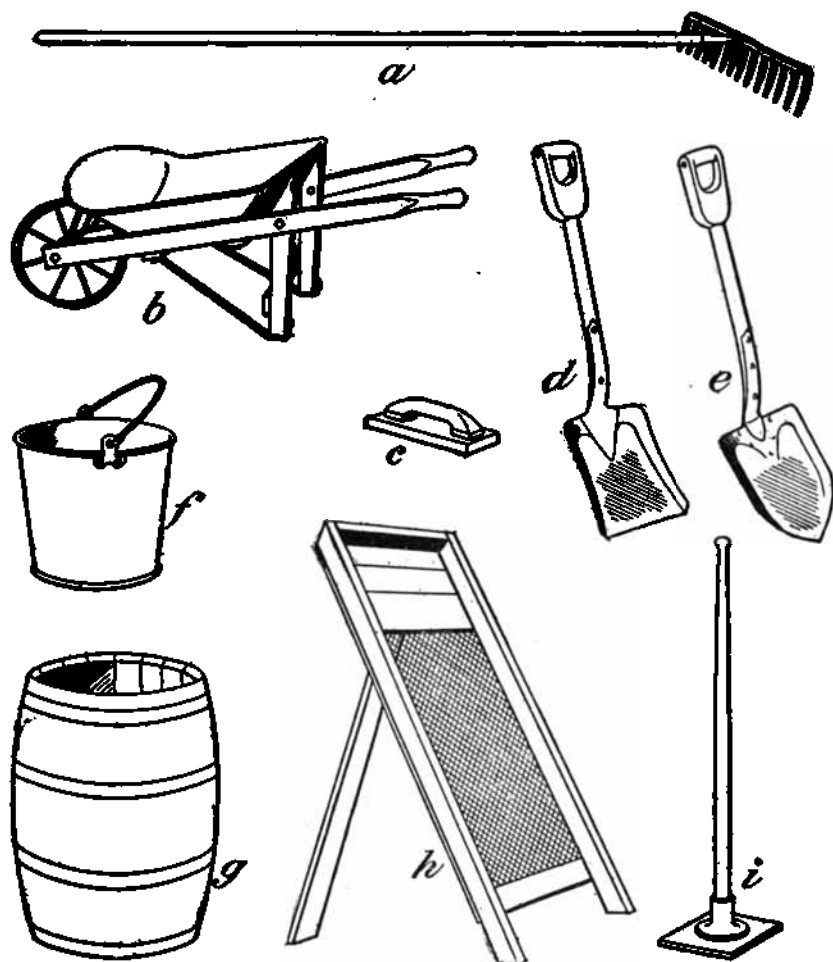
FIG. 213.—Tools used in making concrete on the farm. a, Rake; b, wheelbarrow; c, wooden float; d, square-nosed shovel; e, round-nosed shovel; f, bucket; g, water barrel; h, gravel screen; i, tamper.—U. S. Dept. of Agriculture.
