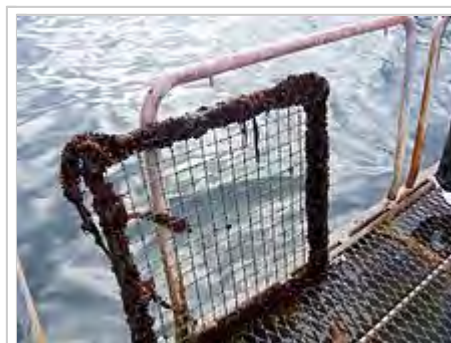
Section of a fish net on a salmon farm near Puerto Montt, Chile. The copper alloy woven mesh inside the frame has resisted biofouling whereas PVC (i.e., the frame around the mesh) is heavily fouled.
