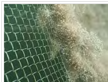
There is no biofouling on a copper alloy mesh after 4 months immersed in the waters of the North Atlantic (foreground), whereas hydroids have grown on high-density polyethylene tubing (background).
