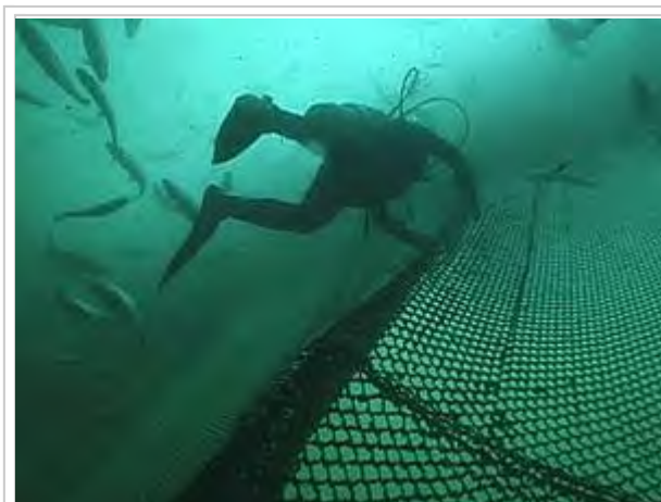
A copper alloy pen that has been deployed on a fish farm at depth of 14 feet for one year shows no signs of biofouling.
