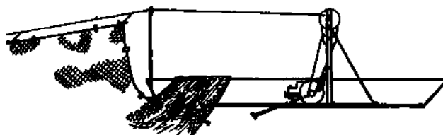
Fig 548 Motorized hauling of the wing of a seine net with an additional line as operated in Germany (1939).
