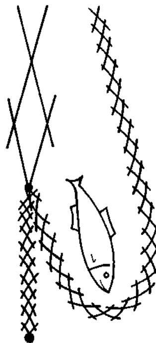
Fig 715 Principle of catching in two-walled netting. (T Mengi, 1977).
