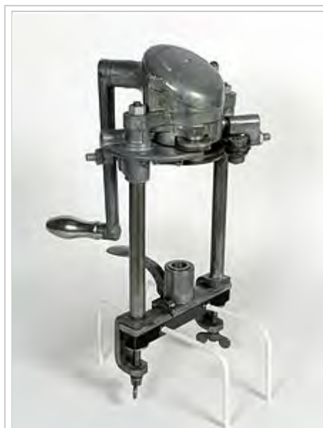
A Dixie Can Sealer for home use. Now in Thinktank, Birmingham Science Museum.
