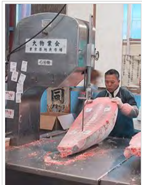
Cutting frozen tuna using a bandsaw in the Tsukiji fish market in Tokyo, Japan (2002)
