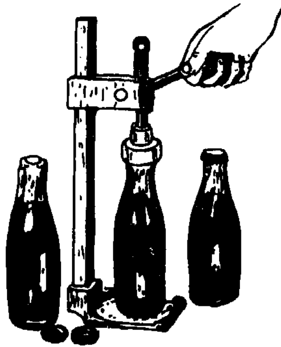
figure 10: A metal bottle top sealer
