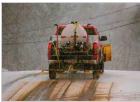
Picture of truck applying liquid de-icer (magnesium chloride) to city streets.
