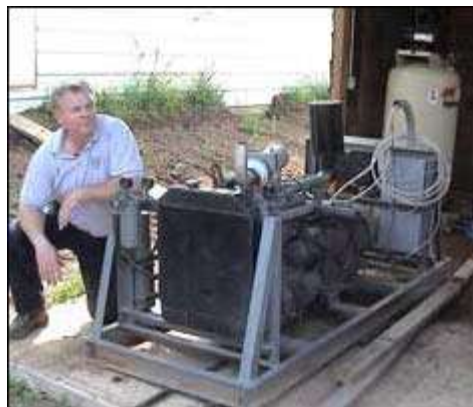
Figure 10: 15 kWe Used Oil Genset (Renewable Oil International)
