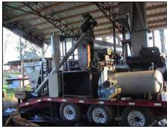
Figure 9: 5 TPD Bio-Oil Pilot Plant (Renewable Oil International)
