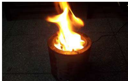
Figure 7b: Oil soaked MSW stove test
