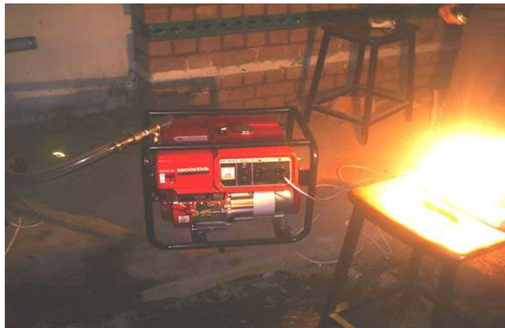
Figure 9 Synthesis Gas Operating the Engine
