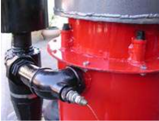
Newly combined cyclone and packed bed filter
