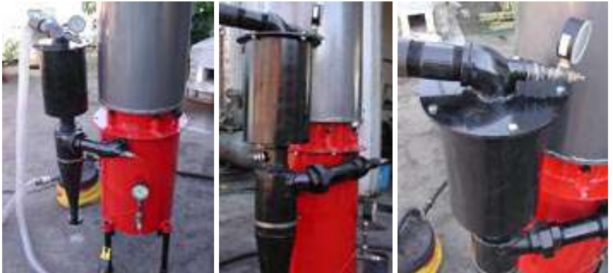
Newly combined cyclone and packed bed filter
