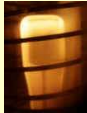
One inch birch dowell pyrolysing at 600C
