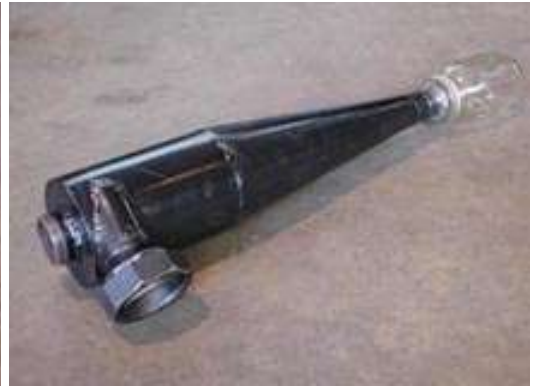
Air preheating / syngas cooling stainless steel heat exchanger
