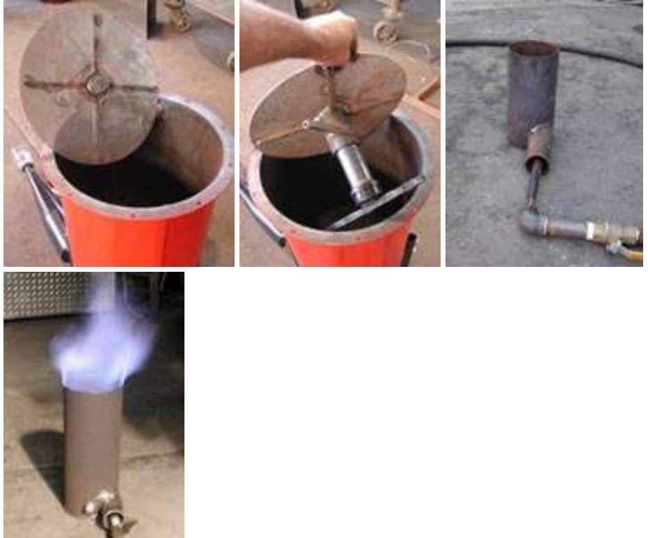
Rotary ash grate, gas cowling and swirl burner
