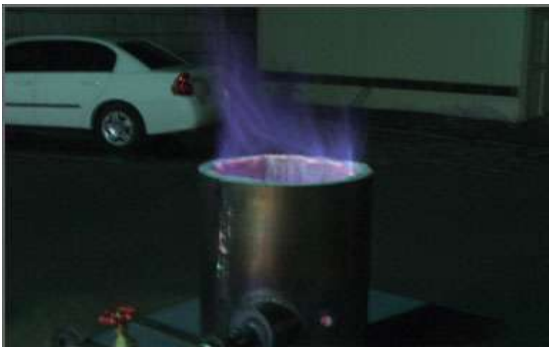
Clean hydrogen flame, invisible during daylight.
