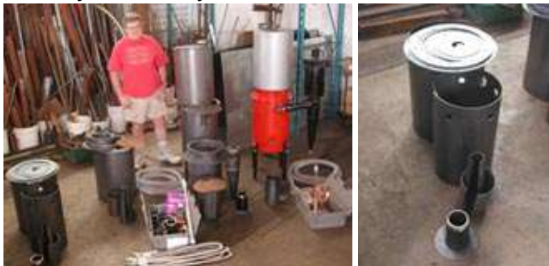
GEK kit at various levels of part count, welded state, and assembly/disassembly
