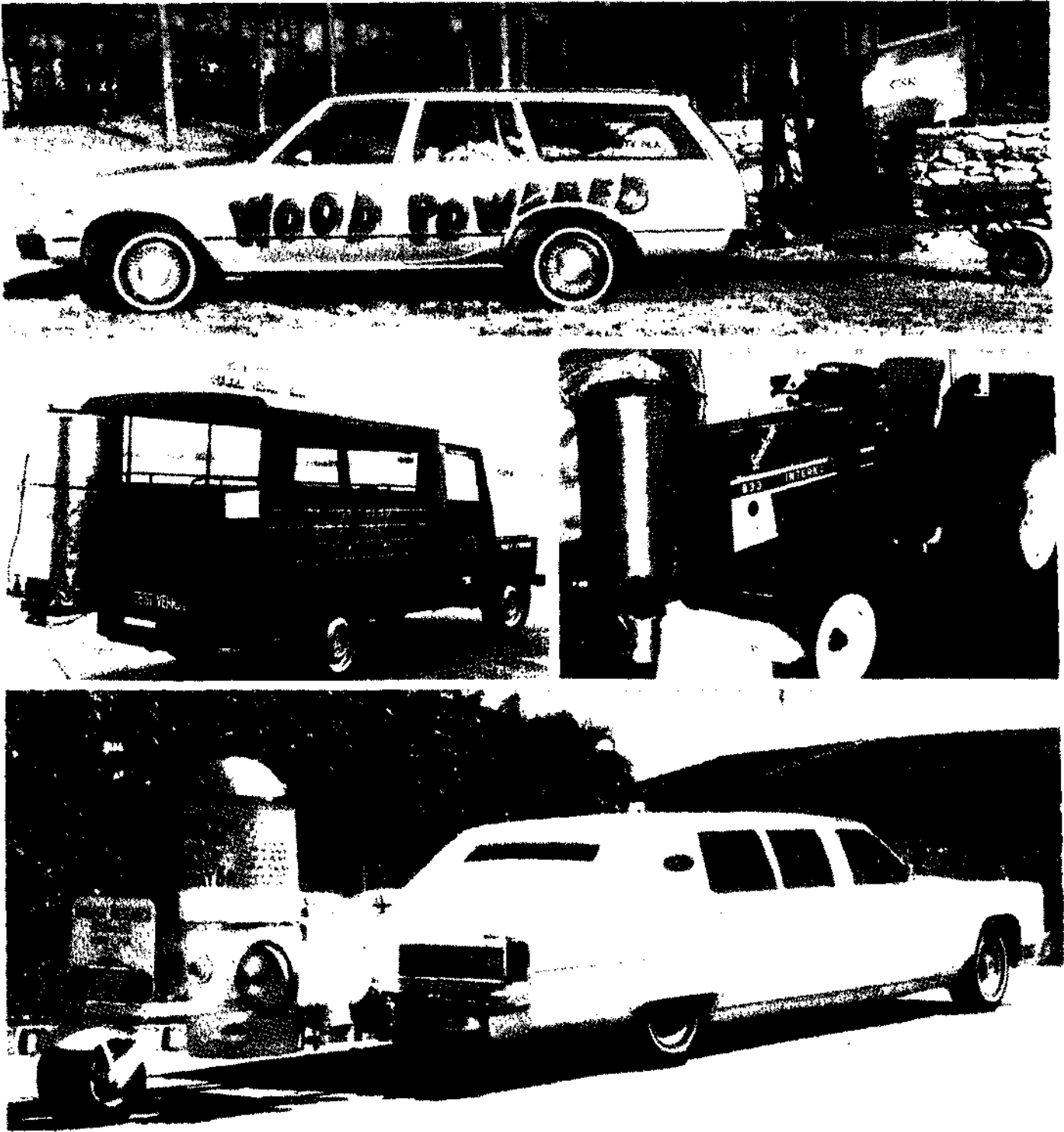
Fig. 2.2. Vehicle gasifiers after OPEC (Source: NAS 1983)
