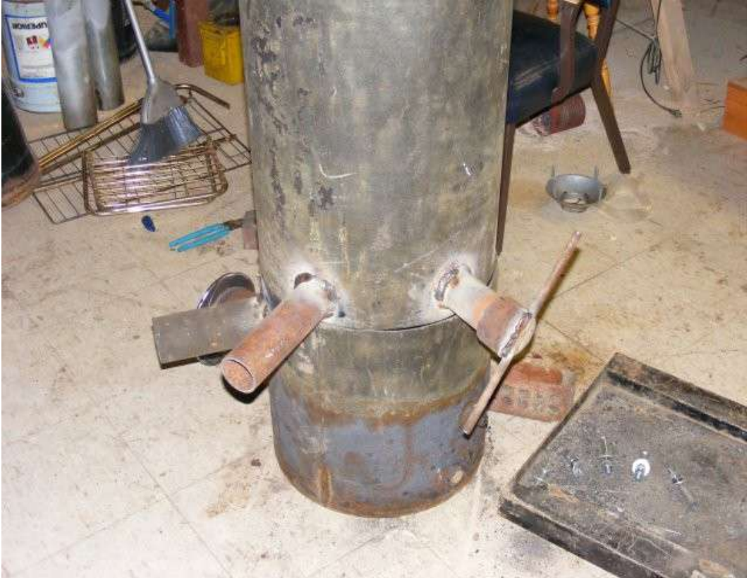
Fitting tank together. using a rope gasket to seal tank.
