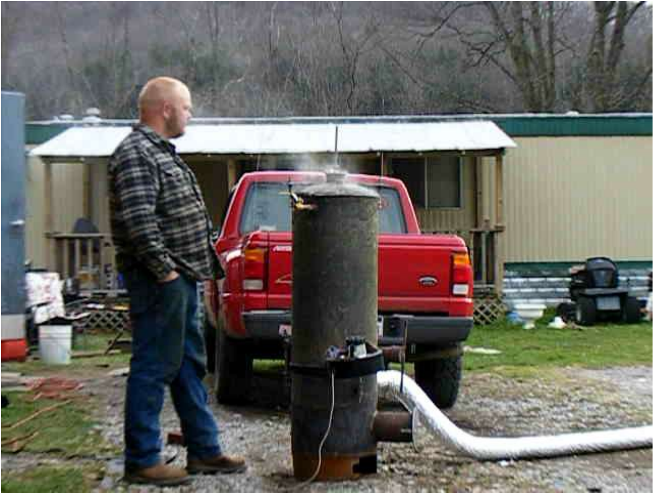
Full view of the gasifier operation. No steam or smoke anywhere else. The flex pipe is also pulsing at this point. Found this to be normal as I was a bit worried about it. Blower is on very low speed.
