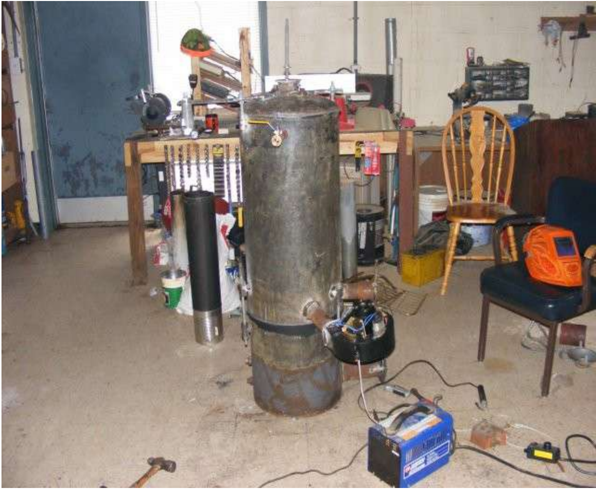
Gasifier completed. Waiting to make charcoal.
