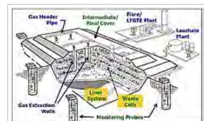
A layout of landfill gas collection system. [9]
