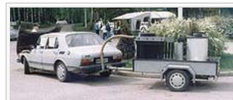
Saab 99 running on wood gas in Finland. The gas generator is on the trailer. [ edit ]
