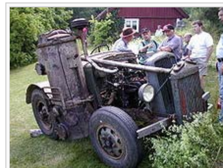
Wood gasifier on a Ford truck converted to a tractor
