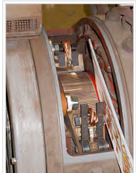
Different types of brushes have different brush contact angles [6]
