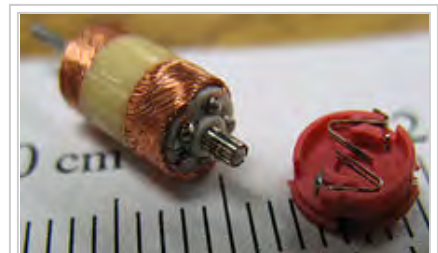
A tiny 5-segment commutator less than 2 mm in diameter, on a direct-current motor in a toy radio control ZipZaps car.
