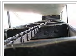
Interior view of silo unloader conveyor paddles and drive chain.
