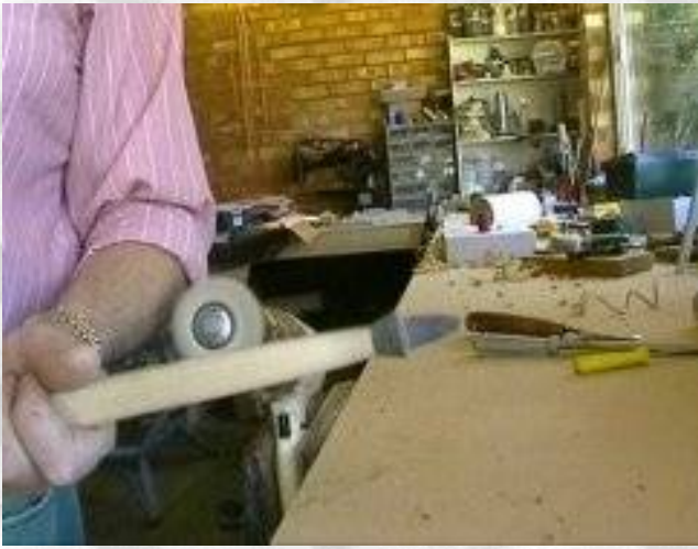
The unpolished fully shaped nock
