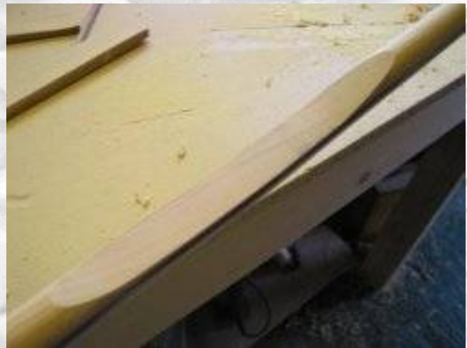
Planed handle before a leather grip is fitted.
