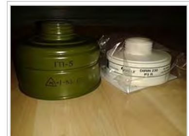
An asbestos containing Russian GP-5 filter and a safe modern one in comparison.
