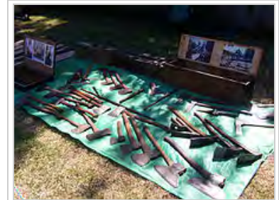
A collection of old Australian cutting tools including broad axes, broad hatchets, mortising axes, carpenter's and felling axes. Also five adzes, a corner chisel, two froes, and a twibil
