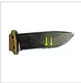
The Gerber LMF II ASEK used to sever the 220 volt line; arrows point to the minor damage done to the cutting edge by the current.
