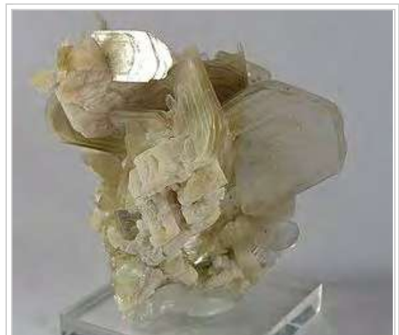
Muscovite, a mineral species in the mica group, within the phyllosilicate subclass
