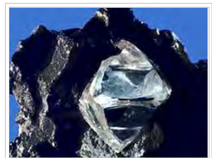
Diamond is the hardest natural material, and has a Mohs hardness of 10.
