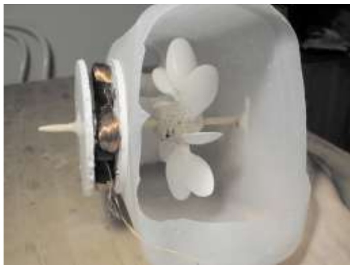
The completed micro-hydro turbine.
