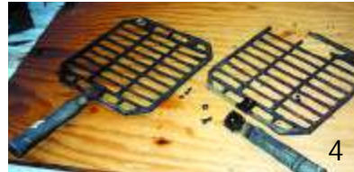
4. Old Hibachi grills were used for the deflection plate in the culvert dam.
