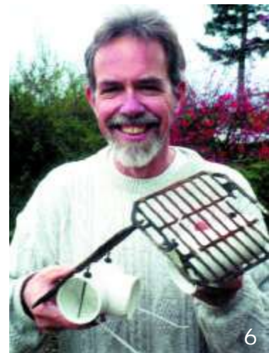
6. The grills are fastened to the 2-inch intake tees with plastic ties.
