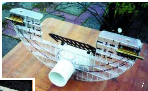
7. The culvert dam for the south culvert is ready to install.
