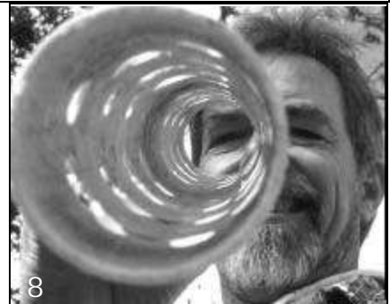
8. Inside view of the 2-inch filter core after drilling.
