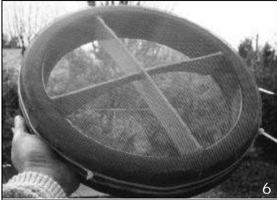
6. Plastic ties hold the brass screen to the lid.
