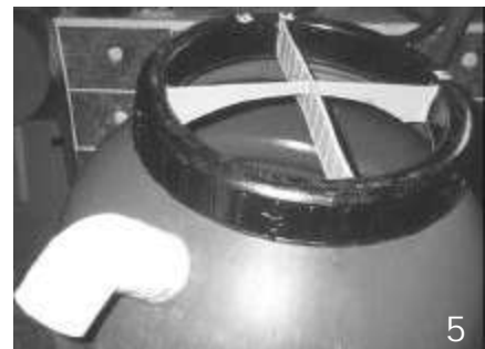
5. Ribs added to the threaded ring help support the brass screen.
