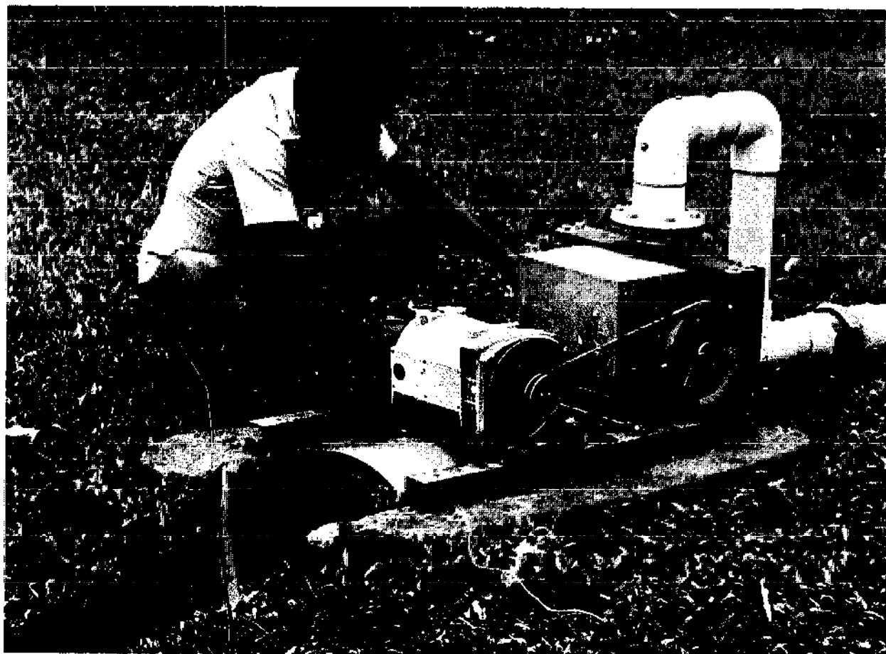
A 5 kW Pelton prototype designed at the Appropriate Technology Development Institute (Lae, PNG) for local fabrication and quick, trouble-free installation. A box can be used to protect the equipment from the elements.
