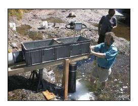
The LH1000 is an exciting hydro turbine that produces DC electrical power at sites with sufficient water flowing across relatively level terrain. The LH1000 uses a durable, low-head bronze propeller to produce power on a head of 2 to 10 feet. At 10 ft of head, the output from this turbine is <u>one kilowatt</u>, which is enough to supply the electrical requirements for an average household.
