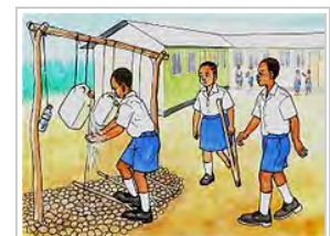
Drawing of a tippy tap with soap for hand washing at a school (Tanzania)
