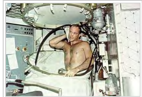
Astronaut taking a hot bath in the crew quarters of the Orbital Workshop (OWS) of the Skylab space station cluster in Earth orbit. In deploying the shower facility the shower curtain is pulled up from the floor and attached to the ceiling. The water comes through a push-button shower head attached to a flexible hose. Water is drawn off by a vacuum system.
