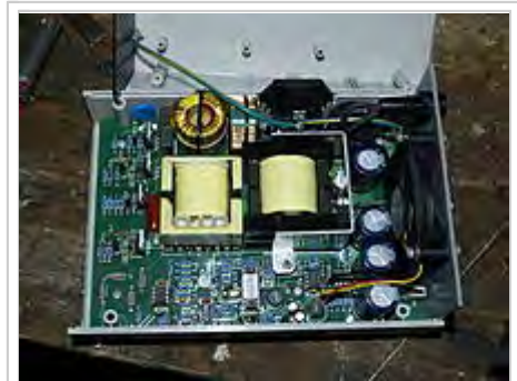
Inside an SWEA 250W transformer-coupled grid-tie inverter
