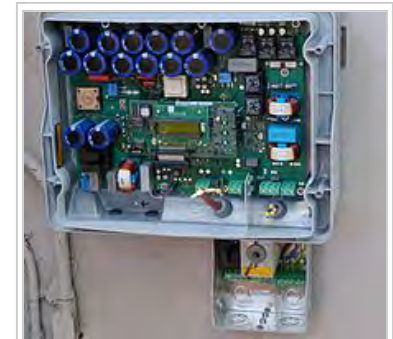
Internal view of a solar inverter. Note the many large capacitors (blue cylinders), used to store energy briefly and improve the output waveform.
