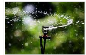
Impact sprinkler head
