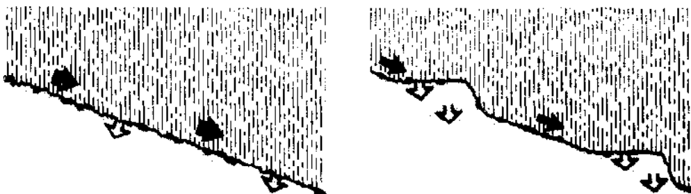
Fig.8 Run-off interception with ridges
