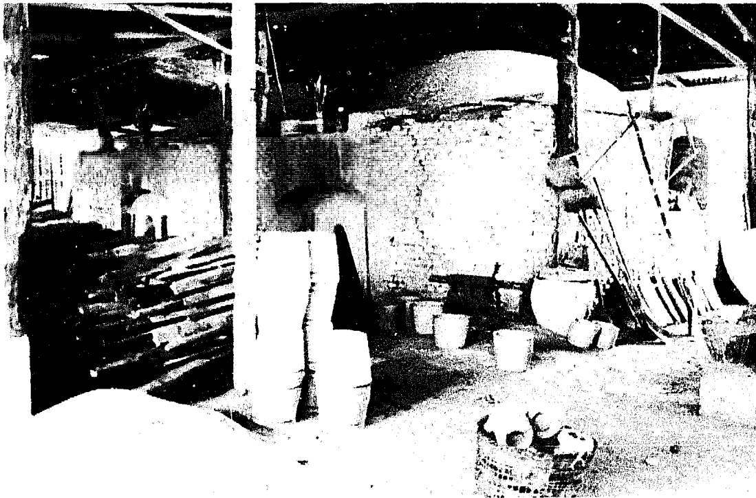
Fig. 2-27: Two wood-fired kilns seen from firebox side
