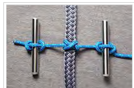
A constrictor knot prepared for tightening using two metal rods and marlinespike hitches
