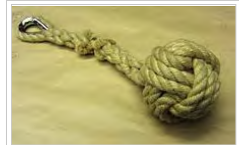
a monkey's fist with an eye splice, custom-made at the chandlers Arthur Beale
