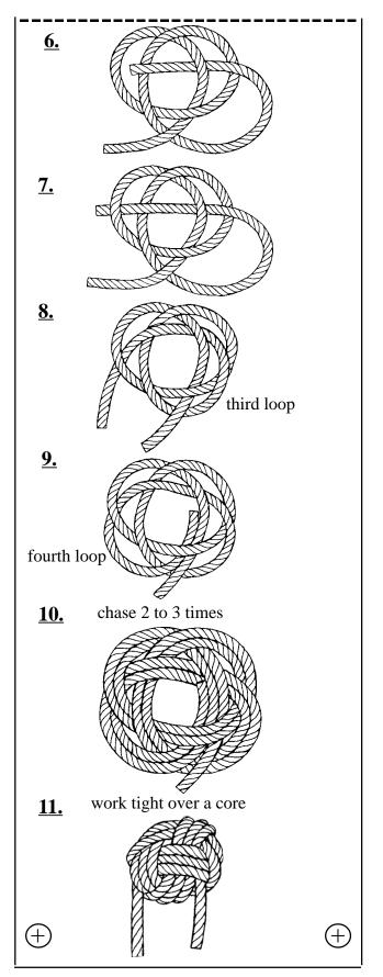
finally under the left side of the of the bottom loop. (8) Pull the running end through until a third loop equal in size to the first two loops. (9) Add the fourth loop by placing the running end parallel to the standing end. (10) Chase the original pattern 2 to 3 times. (11) Work tight over the core.
