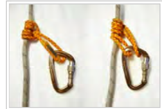
A Prusik (left) and Autoblock (right). Both are used as rappel backups.
