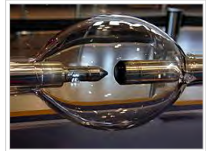
15 kW xenon short-arc lamp used in IMAX projectors
