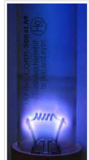
Germicidal lamps are simple low-pressure mercury vapor discharges in a fused quartz envelope.
