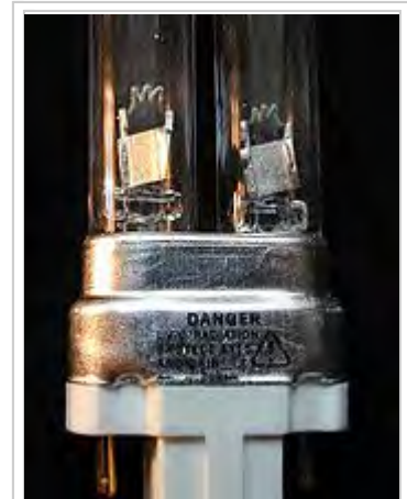
Close-up of the electrodes and the safety warning
